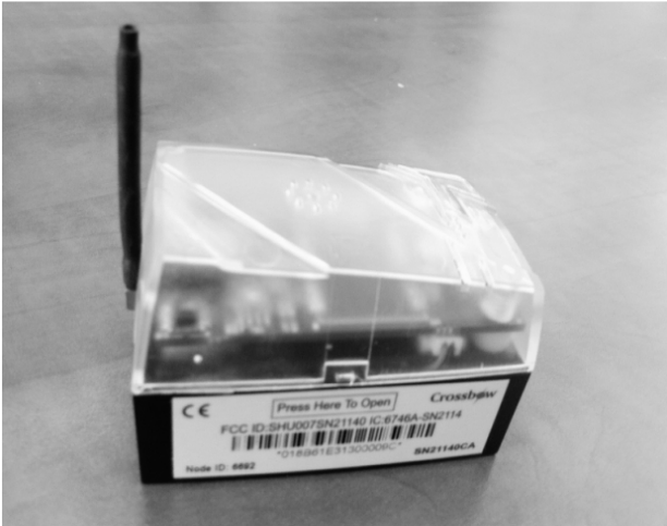
Fig. 6 – Wireless network node equipped with MTS400 sensor
