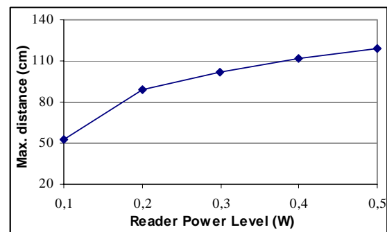
Fig. 13 – Max. distance of tag detection vs. radiated power
