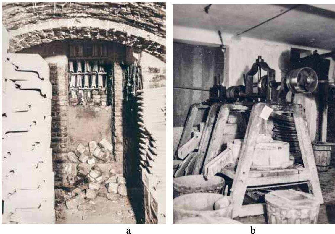
Figure 6. – I. Levynsky's factory: a – kiln for baking a tile (Klimashevskiy, 2020, p. 166); b – press in the tile department of I. Levynsky's factory (Klimashevskiy, 2020, p. 168).
