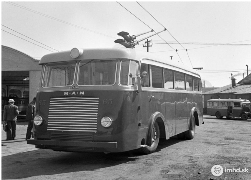
Figure 5. MAN MPE 4500 I/Sodomka/SSW trolleybus produced in 1940 with current collectors mounted on one axle in Bratislava (then Czechoslovakia) (Popis typu vozidla..., n. d.).
