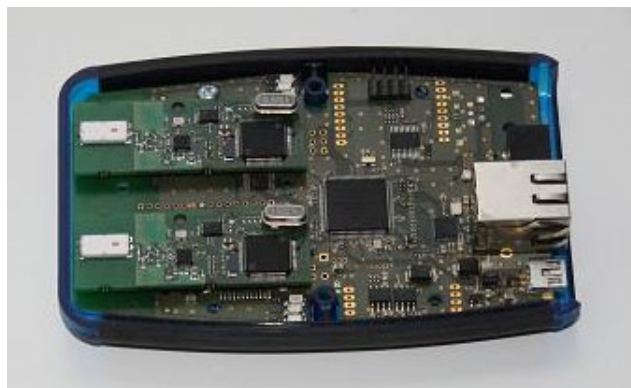
Fig. 4 – PCB for gateway platform
