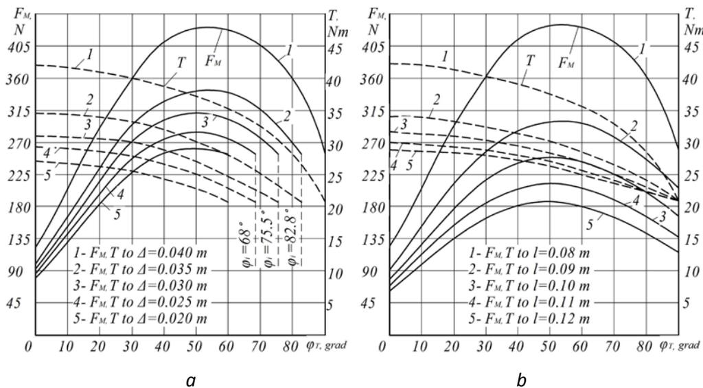
Fig. 3. Characteristic curves of torque  $T$  and additional moving force  $F_M$  at rotation of a group of scrapers depending on: a -  $\Delta$ ; b -  $l$  and the value of  $\varphi_T$
