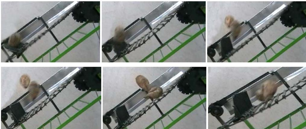
Fig. 7. A photographic shooting sheet of the conducted experiments aimed at the determination of the trajectory and the distance of root crop flying
