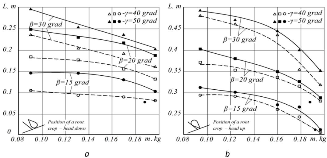
Fig. 8. Flying distance of root crops  $L$  until their second interaction with belt bars-vs-beet root mass  $m$  curves at various positions of a root crop: a – head down; b – head up
