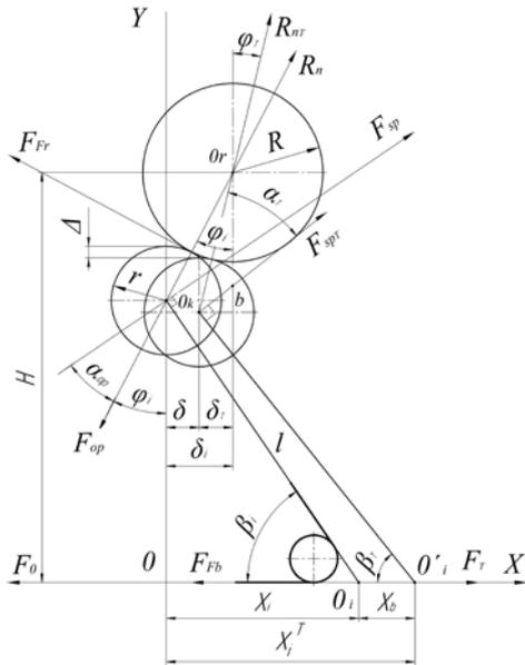
Fig. 2. Scheme of Determining Interaction Parameters of a Roller and a Cam
