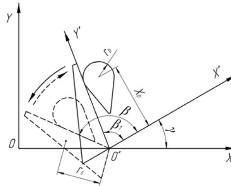
Fig. 4. Pattern of root crop motion along the surface of a scraper
