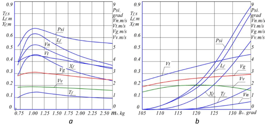
Fig. 5. Change in parameters of root crop throwing depending on: a – mass  $m_b$ ; b – an angle of deflection of a scraper  $\beta$
