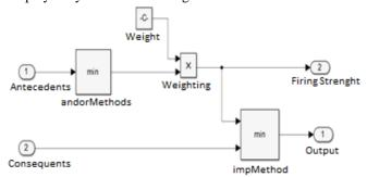
Fig. 7. Scheme for handling incoming fuzzy values using the rule "if-then".
