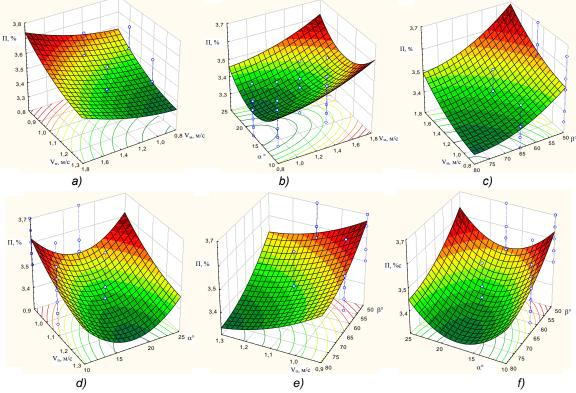
**Fig.7 – Response surfaces of damage** D**, % of root crops from** a):  $D = f(V_c, V_c); b$ ):  $D = f(\alpha, V_m); c$ ):  $D = f(\beta, V_m); d$ ):  $D = f(\alpha, V_c); e$ ):  $D = f(\beta, V_c); f$ :  $D = f(\alpha, \beta)$
