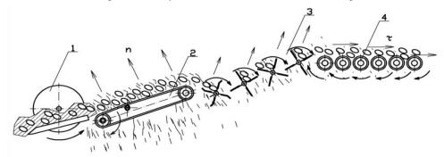
Fig.1 – Root crop and potato cleaning system
