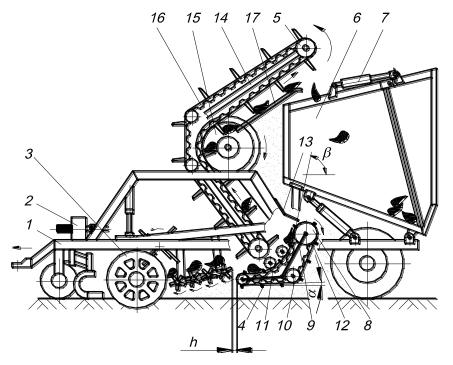
Fig.3 – Design and process flow sheet of a semi-trailing root crop harvester 1 – frame; 2 – transmission; 3 – digging wheels; 4 – intake two-element separating conveyor; 5 – loader conveyor; 6 – hopper; 7 – hydraulic system; 8 – driving drums; 9 – frame of intake conveyor; 10 – bottom rolls; 11 – bearing rollers; 12 – canvas; 13 – casing; 14 – frame of a loader conveyor; 15 – drum; 16 – canvas;17 – guide grid
