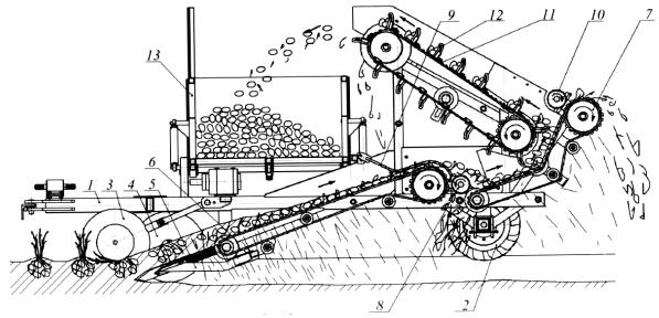
**Fig.2 – Design and process flow sheet of a potato harvesting machine** 1 – frame; 2 – running wheels; 3 – track roller; 4 – cut off disk; 5 – shares; 6 – intake conveyor; 7 – transmission L-shaped conveyer; 8 – receiving roll; 9 – top separator rods; 10 – beater roll; 11 – loader conveyor; 12 – scrapers; 13 – hopper
