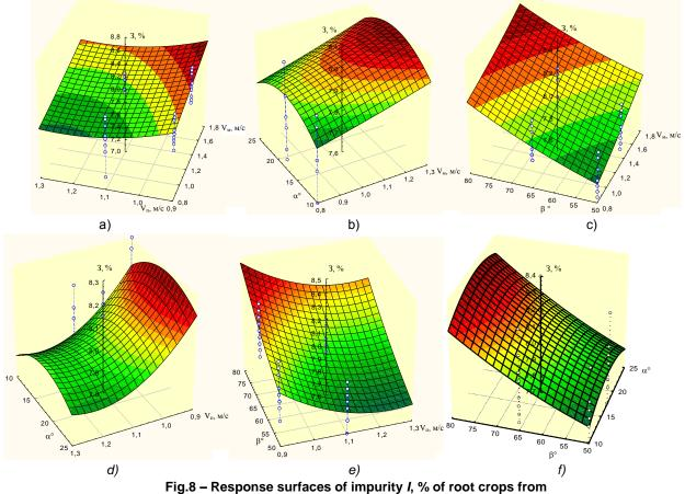
a):  $I = f(V_c, V_m); b): I = f(\alpha, V_m; c): I = f(\beta, V_m); d): I = f(\alpha, V_c); e): I = f(\beta, V_c); f): I = f(\alpha, \beta)$
